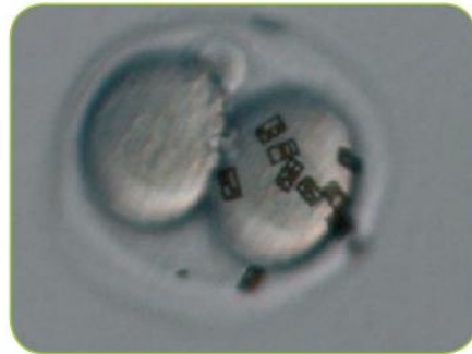
Fig. 3. Light microscope micrograph of a mouse embryo at the two-cell stage with different polysilicon barcodes adhered to the zona pellucida. Picture was taken with a 20x objective on in inverted optical microscope.
